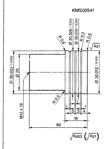
Drill jig for bushing in commutator end shield: to be improvised
